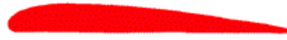
Low camber — low drag — high speed — thin wing section Suitable for race planes, fighters, interceptors, etc.
