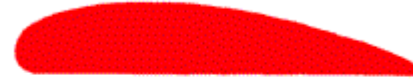
Deep camber — high lift — low speed — thick wing section Suitable for transports, freighters, bombers, etc.
