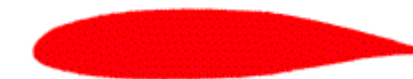
GA(W)-1 airfoil — thicker for better structure and lower weight — good stall characteristics — camber is maintained farther rearward which increases lifting capability over more of the airfoil and decreases drag.
