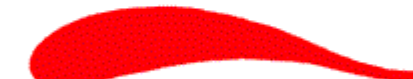
Low lift — high drag — reflex trailing edge wing section. Very little movement of centre of pressure. Good stability.
