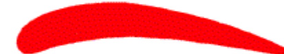
Deep camber — high lift — low speed — thin wing section Suitable as above.
